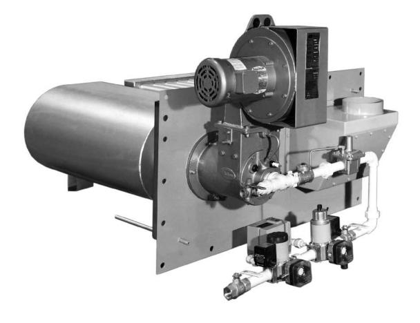
Eclipse Recirculating High Temperature (RHT) indirect air heating burners are designed to heat recirculating ovens and dryers where the products of combustion must be isolated from the process air stream. They are also excellent for use in industrial space heating systems. These burners feature an industry-proven burner, firing chamber and exhaust tubes assembled as a single unit for easy installation and optimum performance.
